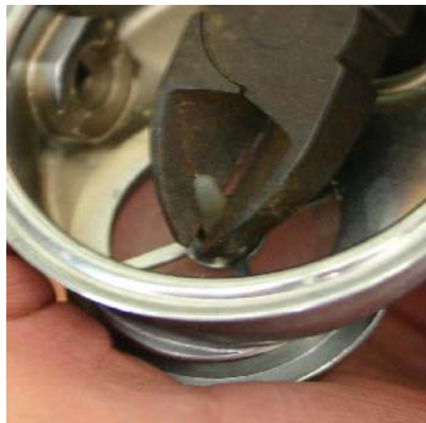
For many second stages it is required to cut of the slack of the exhalation valve once you have it in place, otherwise the part sticking inside the second stage could interfere with membrane movement.
