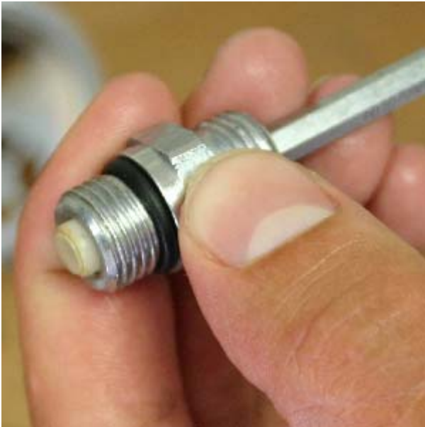
The movable orifice (with the seat) is put in the manufacturer specified position. The technician either knows how many turns he needs to put it in position, or uses an instrument to measure the correct position.
