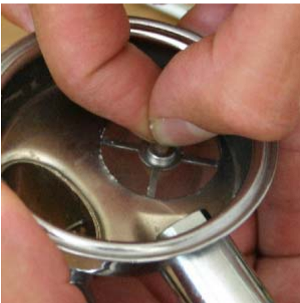
For many second stages it is required to cut of the slack of the exhalation valve once you have it in place, otherwise the part sticking inside the second stage could interfere with membrane movement.
