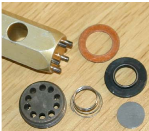
The parts of a second stage inlet valve including the special tool needed for assembly and disassembly.
