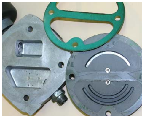
A laminated plate (right) holds both the inlet and the outlet valve for the first stage of modern compressors. It is simply mounted between the cylinder head (left) and the cylinder. Air integrity is assured by adding sealing material (top).
