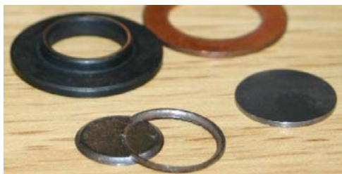
If an outlet valve is malfunctioning, in most cases that is because the seat has cut through the valve as shown on the picture. In that case the valve and washer (the two parts on the right) must be replaced.
