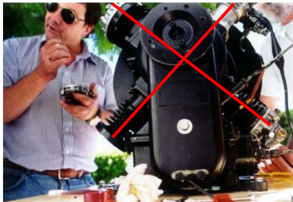
X-shaped compressors have 4 cylinders mounted in the shape of an X. The second stage is mounted opposite the first stage and the fourth stage opposite the third stage.
