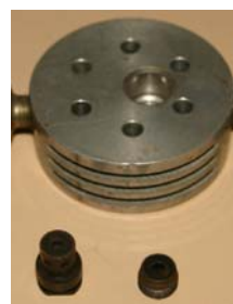
The valves of the last stage are smaller and can't be disassembled.
